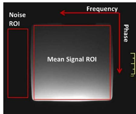
**Figure 15.** Image illustrating ROI placement when estimating the mean SNR.
