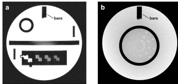
**Figure 4.** Images of slice 1 (a) and slice 11 (b) with the pairs of vertical bars from the 45° crossed wedges indicated. On these images the length difference between the right and left bars is small and typical of well-positioned slices.
