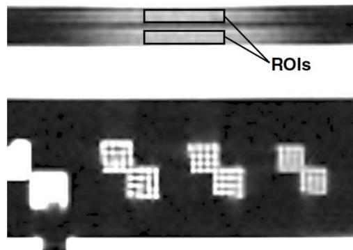
**Figure 7.** Magnified region of slice 1 showing slice thickness signal ramps with ROIs placed for measuring average signal in the ramps.
