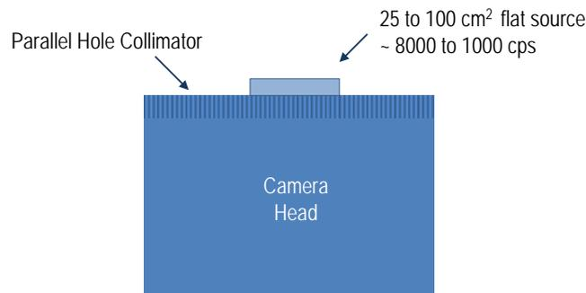
$$\text{System Sensitivity} = \frac{R_{\text{source}}(\text{cps}) - R_{\text{background}}(\text{cps})}{\text{Act}(\mu\text{Ci})}$$
