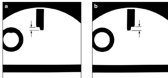
**Figure 5.** Images of slice 1 illustrating measurement of slice position error. The arrows indicate the bar length difference measurement that is to be made.
