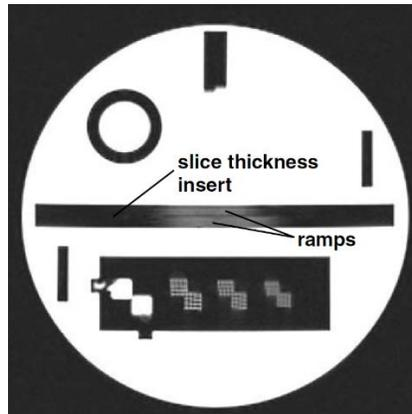
**Figure 6.** Slice 1 with the slice thickness insert and signal ramps indicated.
