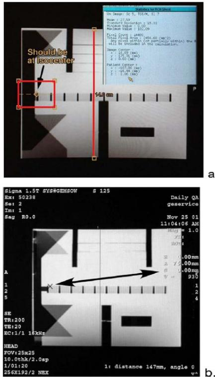
**Figure 3.** a) An example taken from a scanner where a square ROI has been placed with its center on the anterior/superior edge of the grid – exactly where the laser was positioned. In this example the z-coordinate is +1.06. b) An example taken from a scanner and showing the cursor on the superior edge of the grid is exactly at isocenter, S0.00 mm; the S indicates distance from isocenter in the superior z-direction.
