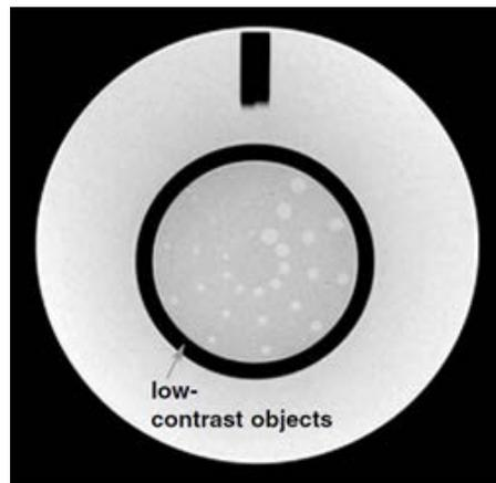
**Figure 12.** Image of slice 11 showing the circle of low-contrast objects for the low-contrast object detectability test.
