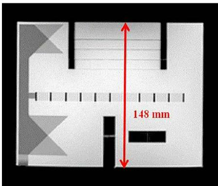
**Figure 8.** Positioning of length measurement on ACR MRI phantom.
