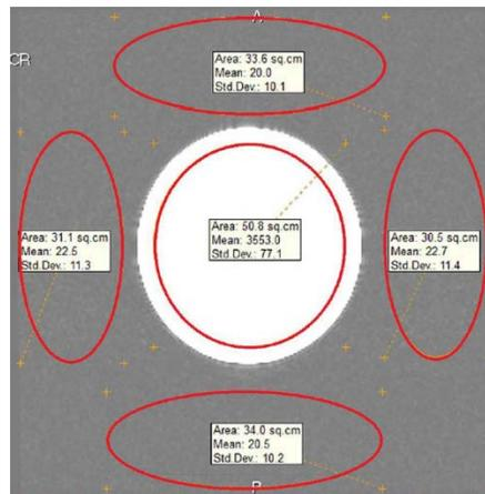
**Figure 14.** Placement of ROIs inside and outside the phantom to determine percent signal ghosting.
