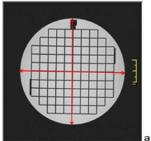
**Figure 9.** Position for x- and y-direction diameter measurements on ACR MRI phantom.
